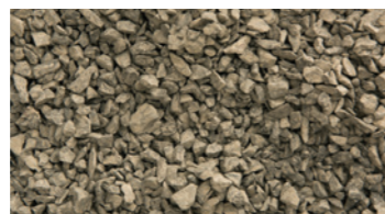
10mm single size drainage aggregate.
