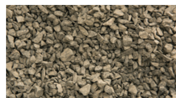
10mm single size drainage aggregate.
